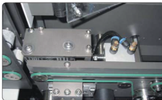
CONTACTLESS DRIVE BY MAGNETIC ROLLER & LM GUIDE POWER TRAIN
