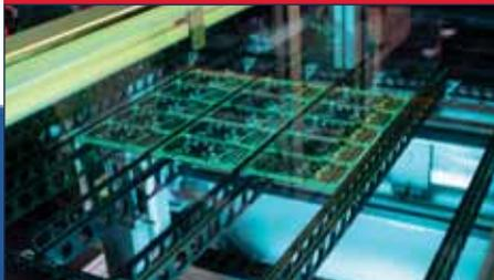
The assemblies are transported strictly horizontally through the soldering system. Furthermore, the PCB is stationary during the soldering process. In this way, components cannot be shifted out of place while the solder is molten. It has thus been possible to eliminate a considerable disadvantage associated with conventional vapour phase soldering systems within which continuous vertical motion of the PCBs is required during soldering. Scrap rates are reduced as a result, as well as costs.
