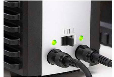
Three position switch. Select left, right or center (both ports operational) to power hand-pieces
