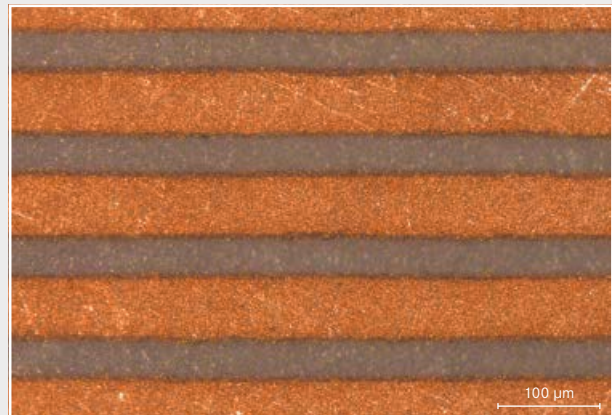
Highly precise structuring of metal layers on ceramics
