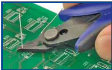
Shearing action of blades produces a clean precise cut with less effort.
